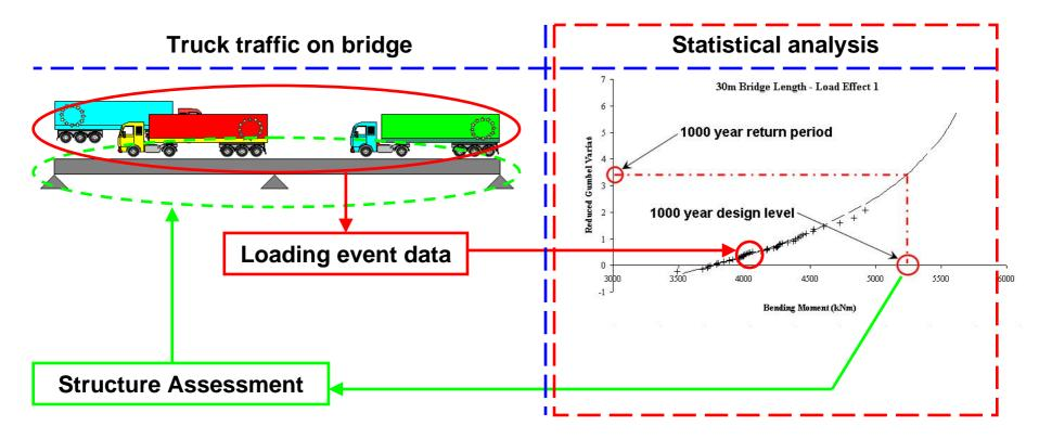
Traffic is generated using Monte Carlo simulation from Weigh-In-Motion data
